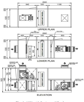
Fig -1: AHU with Desiccant Wheel
