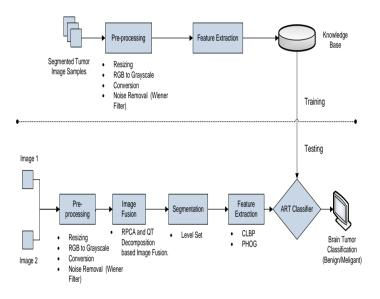
Figure 1 : Proposed Block diagram
