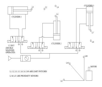
Fig -3: Operation of Pneumatic circuit.
