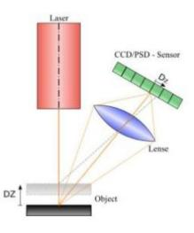
Fig -2: Laser sensor working.
