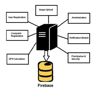
Fig -4.1: Architecture and Modules
