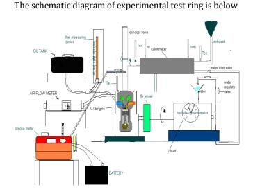
Fig.-1 Schematic diagram of experimental setup
