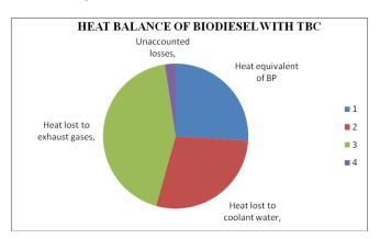
Fig.3:- Heat balance of biodiesel with TBC
