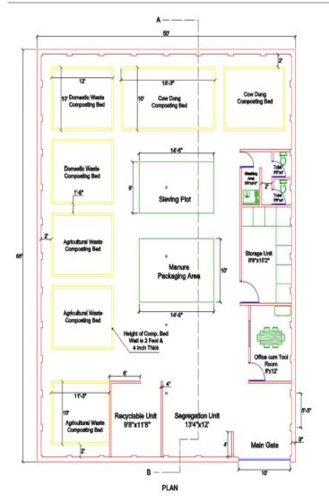
Fig 4: Plan, Elevation & Section for SWM
