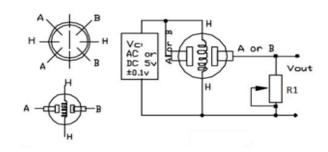
Fig2. Sensor is connected in series with a variable resistor to form a voltage divider circuit
