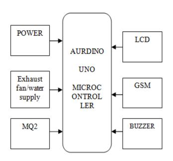
Fig1. Block diagram for gas detection
