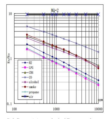
Fig3. Characteristic curve for the different type of gasses.
