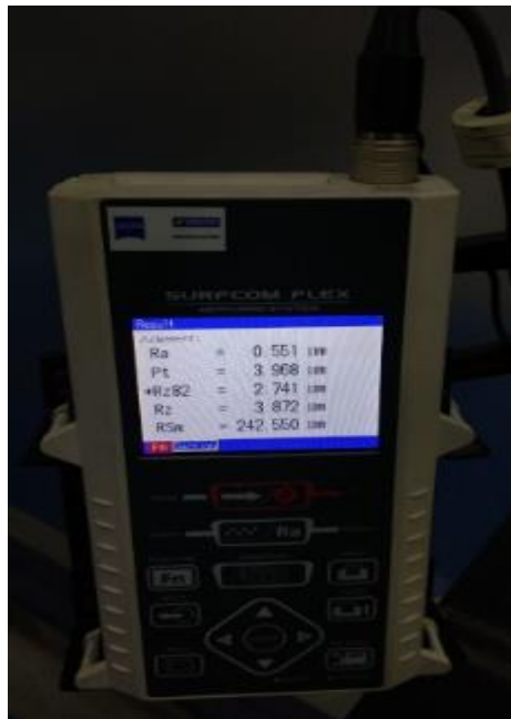
Fig 1.6 Reading of surface roughness
