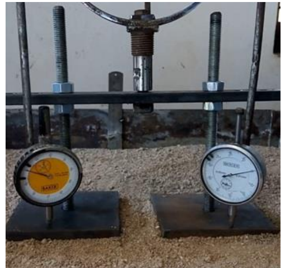
Fig -6: Loading arrangement of two individual footings
