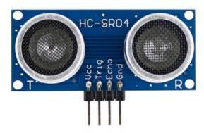
The ultrasonic sensor used here performing function of continuous monitoring of surrounding To detect an obstacle such as human, animals etc.
