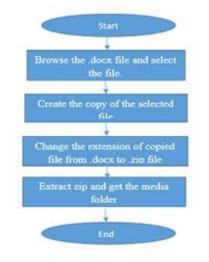
Fig-3: Flow Chart for File Parser Module
