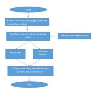
Fig-5: Flow Chart for Selective Encryption Module
