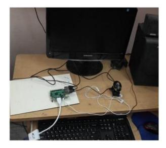
Fig (8) ALPR setup Using Raspberry Pi 3
