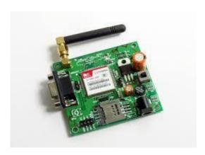
Fig:3 GSM modem
