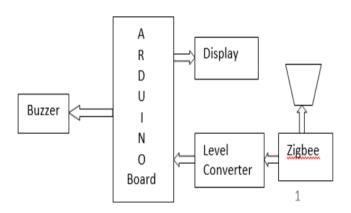
Fig 2. Block Diagram of Receiver Section
