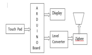
Fig 1. Block Diagram of Transmitter Section
