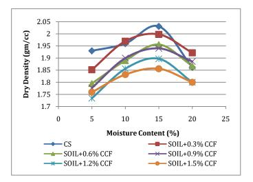
**Chart -1**: Graph of Moisture content v/s Dry Density for soil specimen with varying percentage of CCF
