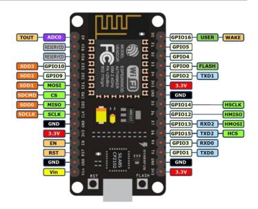
Fig -1: ESP 8266 Pin Diagram
