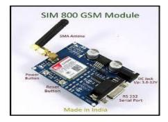
Fig - 3: GSM Module
