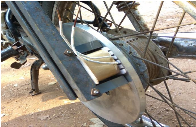
Fig -3: Electromagnet attached near to disc (3mm gap)
