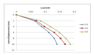
**Chart -7**: Load verses settlement curve for L/D= 40 and inclination= 45°
