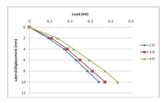
**Chart -6**: Load verses settlement curve for L/D= 20 and inclination= 15°
