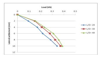
**Chart -4**: Load verses settlement curve for spacing= 2D and inclination= 15°
