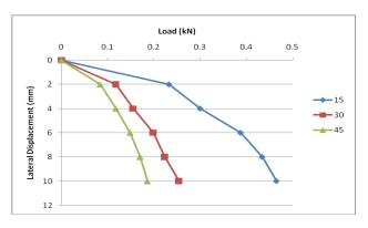
**Chart -9**: Load verses settlement curve for L/D= 40 and spacing= 4D
