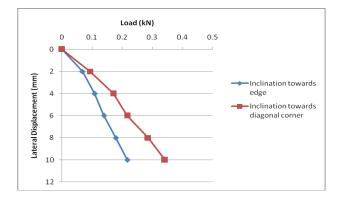
**Chart -2**: Load verses settlement curve for L/D=20, spacing= 2D and inclination= 15°
