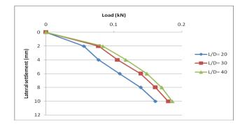
**Chart -5**: Load verses settlement curve for spacing= 4D and inclination= 45°
