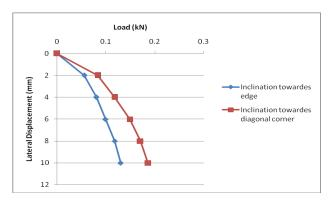
**Chart -3**: Load verses settlement curve for L/D=40, spacing= 4D and inclination= 45°
