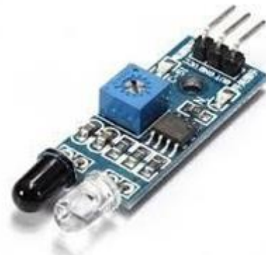
Fig-9: IR Transceiver
