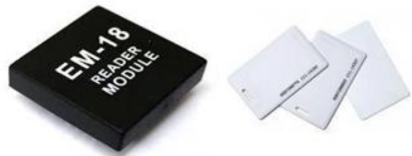
Fig-4: RFID Reader and Tag
