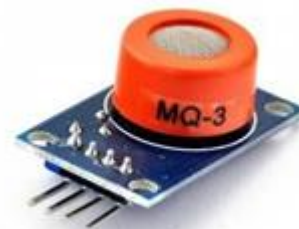
Fig-5: Alcohol Sensor
