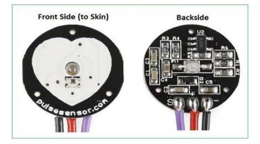
Fig -1: Pulse Sensor
