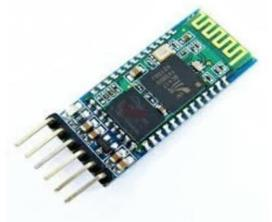
Fig-3: Bluetooth Transceiver Module
