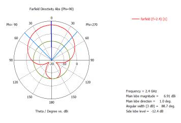
Fig -9: Directivity of paper substrate
