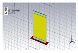
Fig -2: Geometry of rectangular microstrip patch antenna using alumina substrate.
