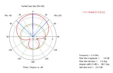
Fig -11: Gain of paper substrate
