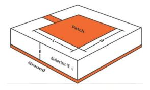
Fig -1: Microstrip patch antenna
