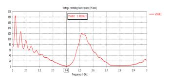
**Fig -6:** VSWR of alumina substrate
