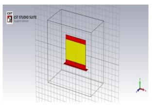
Fig -3:Geometry of rectangular microstrip patch antenna using paper substrate.
