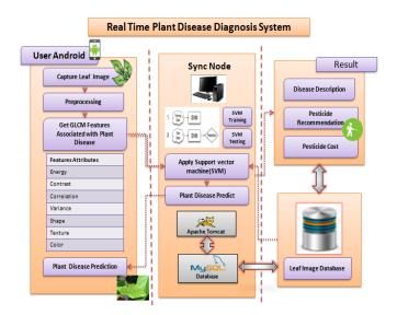
Fig-1: Diagram For Proposed system
