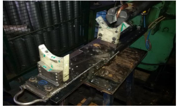
Fig.8. Automated Fixture for Seam Welding Machine
