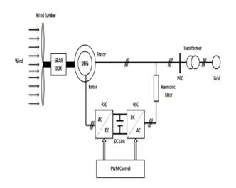
Figure: 1.Basic diagram of DFIG wind turbine
