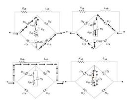
Figure: 5.Bridge Type Fault Current Limiter Operation
