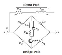
Figure: 4.Bridge Type Fault Current Limiter
