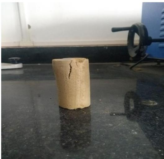
Fig-15: Failed soil specimen
