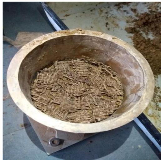
Fig-16: Preparation of sample with jute layers
