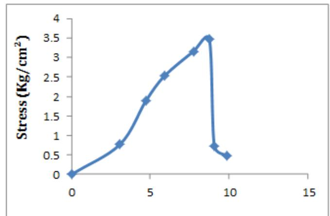
Chart -5: Stress – strain graph for jute layers coated with bitumen placed simultaneously in the sample
