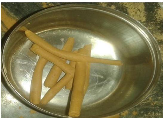
**Fig-7:** Threads of soil in moisture container (test for plastic limit)
