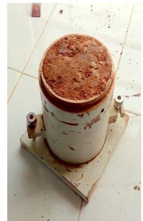
**Fig-10:** Proctor mould with compacted soil
