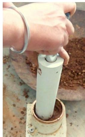
**Fig-9:** Rammering by 2.6 kg rammer
