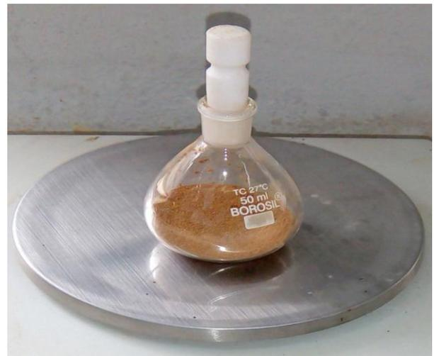
**Fig-8:** Specific gravity test
