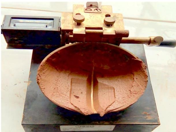
**Fig-6:** Cassagrande apparatus (Test for liquid limit).
