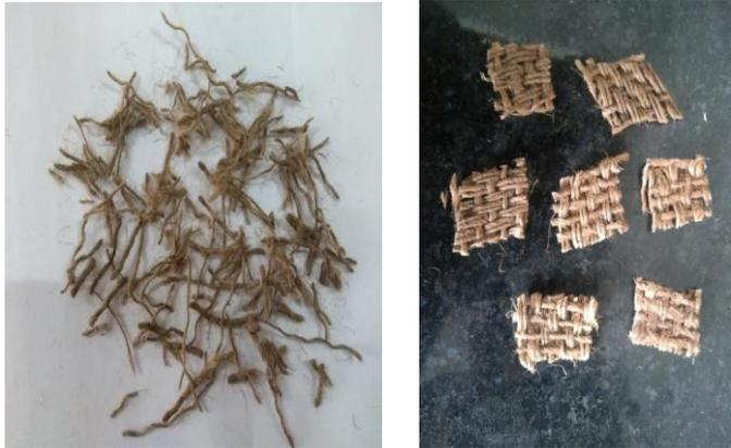
Fig-1: Jute fiber used as reinforcement
