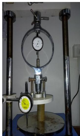
Fig-14: Soil specimen under the plunger
