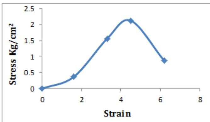
Chart -4: Stress – strain graph for jute layers placed simultaneously in the sample
