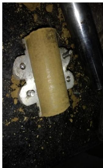
Fig-13: Soil specimen for Ucs test
