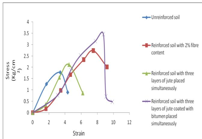
**Chart -6:** Curves showing comparisons of the maximum UCS values for all the cases of unreinforced and reinforced soil sample
