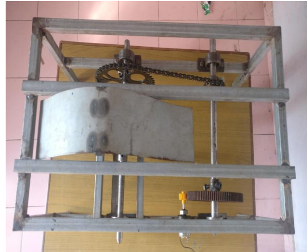
Fig.-2 Experimental Setup of Generation of Power Using Railway Track
