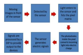
Fig 7: Wave Flow of Touch less Touch Screen
