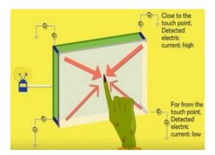
Fig 4: First process of Capacitive Touch Screen
