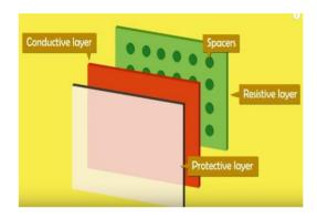
Fig 1: Front View of Resistive Touch Screen Setup
