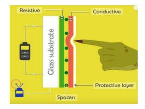
Fig 2: Side View of Resistive Touch Screen Setup
