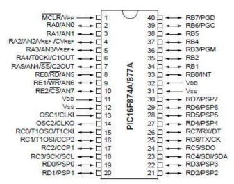
Fig -1: Pin Diagram of PIC16F87A Microcontroller
