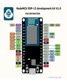
Fig- 3 : Pin diagram of NodeMcu[9]
