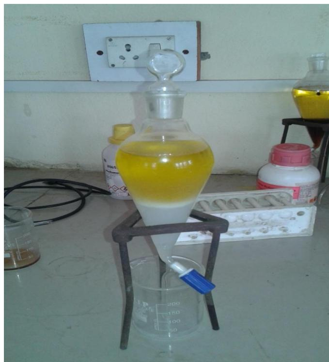
Figure 3.3 Cleansing of Biodiesel
