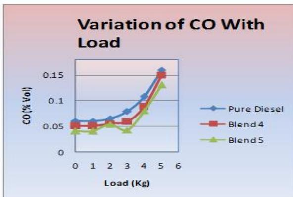
Figure 4.7 Variation of carbon monoxide with Load
