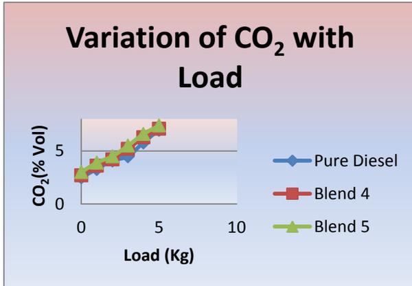
Figure 4.10 Variation of carbon dioxide with Load
