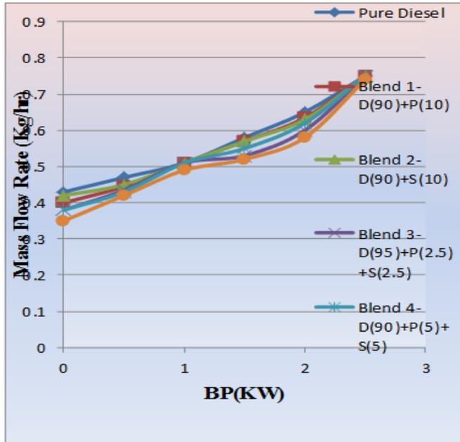
**Figure 4.1 Variation of mass flow rate of fuel with brake power**
