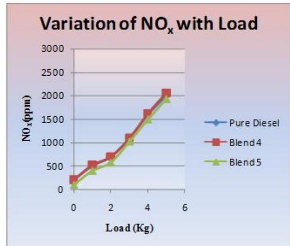
Figure 4.9 Variation of NOx with Load
