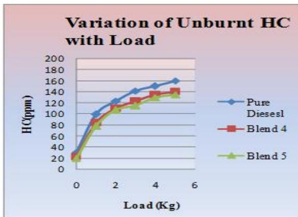
Figure 4.8 Variation of unburnt hydrocarbons with Load
