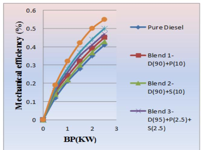
Figure 4.6 Variation of mechanical efficiency with brake power
