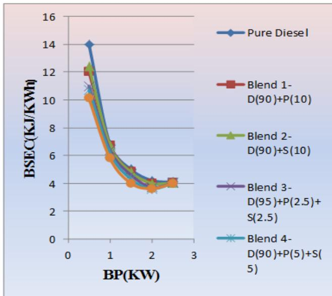
Figure 4.4 Variation of brake specific energy consumption with brake power
