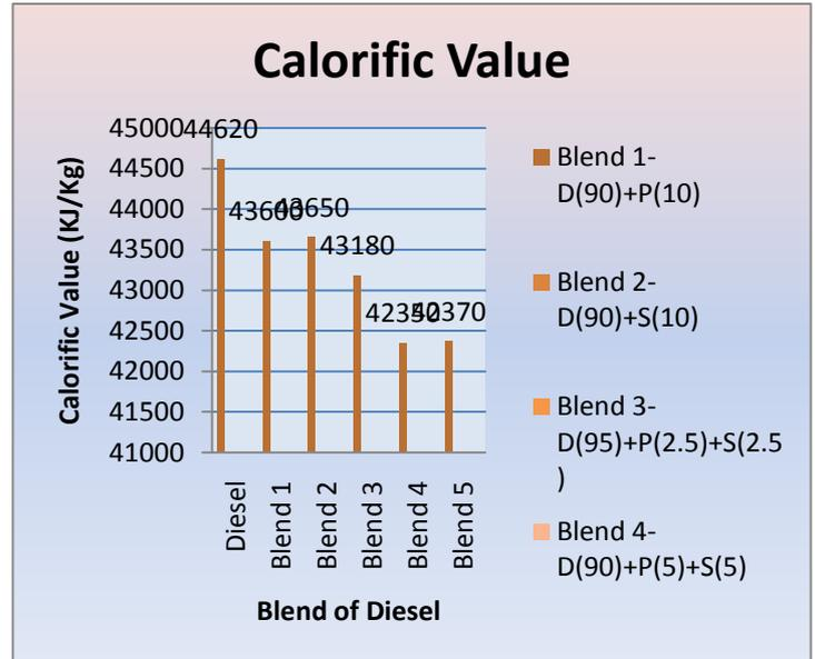
Figure 4.12 Calorific value of biodiesel blends
