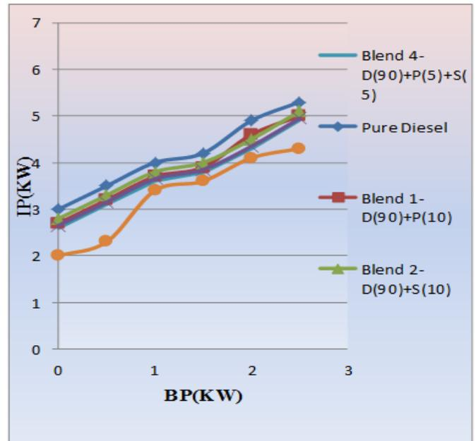
**Figure 4.2 Variation of indicated power with brake power**
