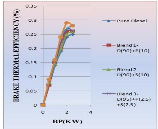
Figure 4.5 Variation of brake thermal efficiency with brake power
