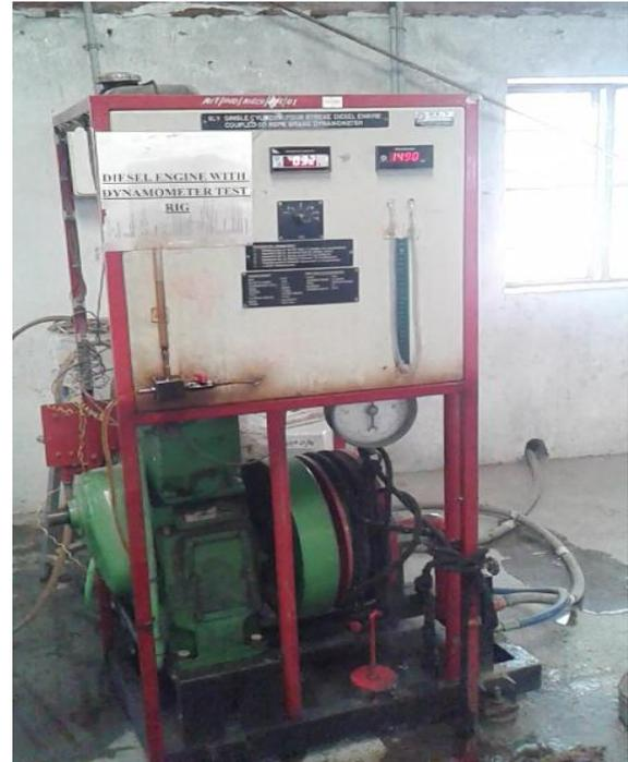
Figure 3.7 The Engine and Dynamometer
