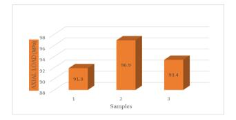
Fig -4: Behavior of two-layer CFRP Wrapped column in transverse orientation under Axial load
