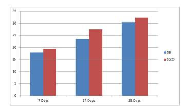
**Graph -1:** Compression between conventional design and 20% replacement for compressive strength.
