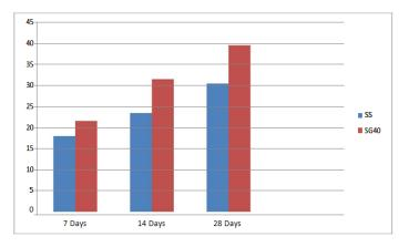
**Graph -2:** Compression between conventional design and 40% replacement for compressive
