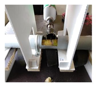
Fig -5.3: Cutting Process of Sugarcane.
