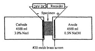
Fig -5.1.1 Schematic diagram of ACMT cell
