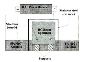
**Fig -3.2**: The set-up used by Azad et al. for accelerating reinforcement corrosion
