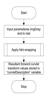
Fig.b : Flow chart of Curvelet Transform
