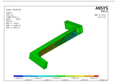
Fig -14 : Beam strengthened at 90 degree oriented sheets at failure
