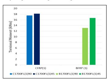
Fig -17 : Comparison of beams wrapped with one layer of CFRP/BFRP oriented at 90 degrees and 45 degrees
