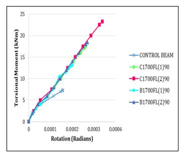
Fig -11: Torsional Moment Vs Rotation Graph of Beams with 90 Degree Oriented Wraps
