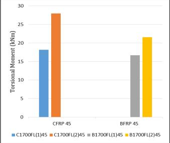
Fig -16 : Comparison of beams wrapped with one layer and two layer of CFRP/BFRP oriented at 45 degrees
