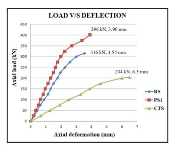
**Chart -1:** Load v/s deflection curves for rebar, PCS and CFST specimens having square geometry
