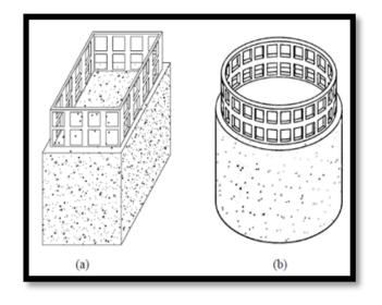
Fig -1: PCS reinforced column
