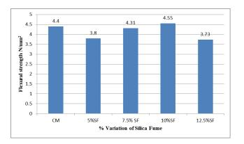
Figure 5: Effect of Silica Fume on Flexural Strength
