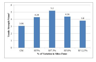
Figure 4: Effect of Silica Fume on Split Tensile Strength Concrete
