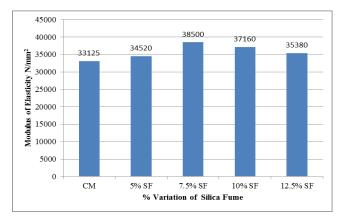
Figure 6 Effect of Silica fume on Modulus of Elasticity
