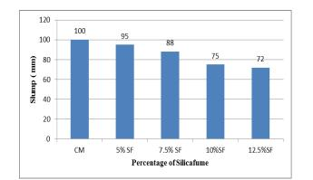
Figure 1: Slump Result of Silica Fume Variation
