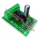
Motor driver ICs act as an interface between microprocessors in robots and the motors in the robot. The most commonly used motor driver ICs are from the L293D.
