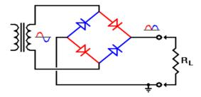
Figure -3: Circuit to step down the voltage from AC to DC
