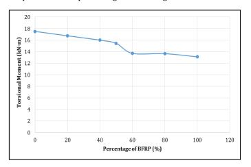
Fig -13 : Replacement of BFRP strips in between CFRP strips
