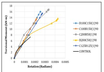
Fig -13 : Torsional Moment Vs Rotation Graph of Hybrid CFRP-BFRP (strips)Beams
