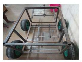
Fig.4 Structural Frame
