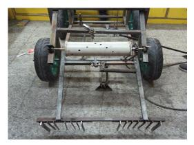
Fig.3 Weeder and Seeder Mechanism
