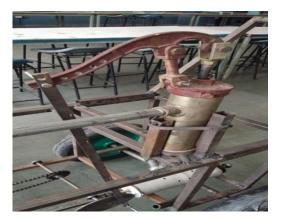
Fig. 2 Slider Crank Mechanism
