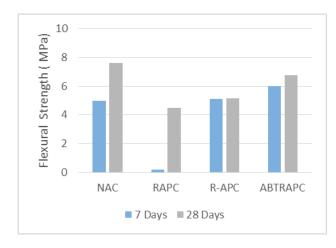
Fig.2. Flexural strength for all mixes
