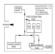
Fig -5: Usage of biogas in Jaggery plant
