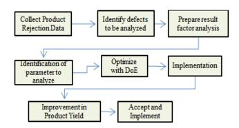
Fig-1: Flow Chart of using Design of Experiments
