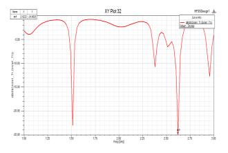
Fig.3. Return loss plot for phase shifter of +20<sup>0</sup>
