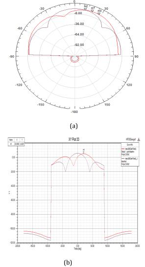
Fig. 4. (a) Radiation pattern (b) Reactangular plot of array antenna with phase shifter of +20<sup>0</sup>
