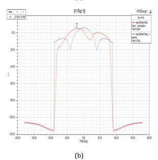
Fig. 6. (a) Radiation pattern (b) Reactangular plot of array antenna with phase shifter of -20<sup>0</sup>
