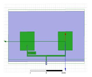
Fig.2. microstrip patch array antenna with transmission line phase shifter of  $\mbox{-}20^{0}$
