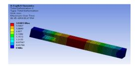
Fig. 3.2 Total deformation non-strengthened beam
