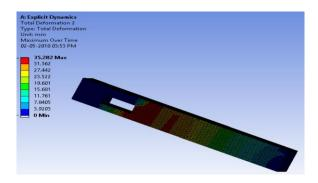
Fig. 3.1 Total deformation non- strengthened beam
