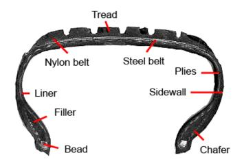
Fig- 2 : Internal structure of Tyre
