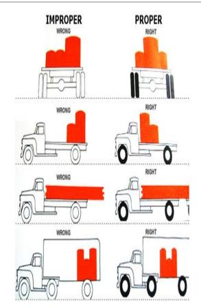
Fig-4 : Loading Diagram
