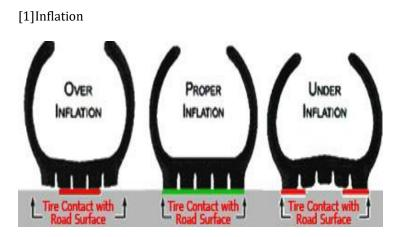
Fig -3 : Effect of inflation on tyre performance
